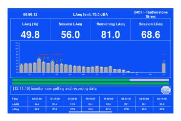
receptors. Live screens change colour to indicate the current sound levels relative to preset limits. A number of limits can be set with time ranges so that the limits automatically change at specific times.
